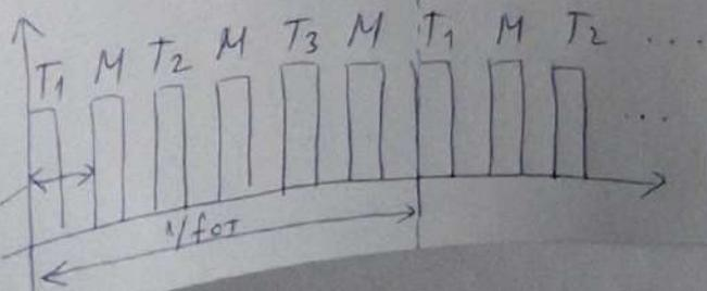
$$T_{MIN} = \frac{1/f_{OT}}{6} = \frac{125 \mu s}{6} = 20.833 \mu s$$
