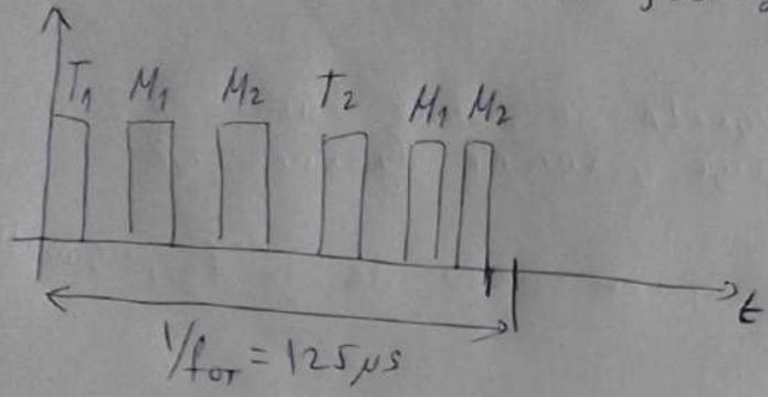
POŠTO SE TELEFONSKI SIGNALI UZORKUJU SAMO PO JEDNOM ( $T_1$  I  $T_2$ ) NJIHOV RASPORED NIJE BITAN. MUZIČKI SIGNALI SE UZORKUJU PO DVA PUTA U TOKU JEDNOG CIKLUSA ( $M_1$  I  $M_2$ ) PA RASTOJANJE (BROJ IMPULSA IZMEĐU) OD  $M_1$  DO  $M_1$  I OD  $M_2$  DO  $M_2$  TREBA DA BUDE FIKSNO.
