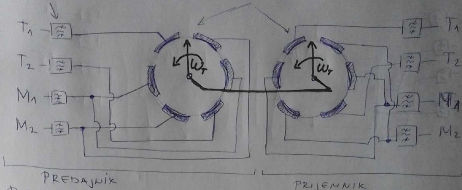
POŠTO SE OBA KLIZAČA OKREĆU ~~ISTO~~ U SMERU SUPROTNOM, KARAKTER NA SATU, RASPORED SIGNALA SHODNO TOME VEZUJEMO NA KONTAKTE. BATO ŠTO IMAMO 6 IMPULSA U TOKU JEDNOG CIKLSA, PRIJEMKI I PREDAJNI DOU IMAJU PO 6 KOLEKTORA, A REDOSLED VEZIVANJA SIGNALA JE ISTI  $T_1, M_1, M_2, T_2, M_1, M_2$ .
