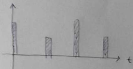
AKO NPR. IMAMO DVA SIGNALA KOJA TREBA DA PRENESEMO PRIMENOM IMPULSNE AMPLITUDSKE MODULACIJE NAJPRE TREBA NA OSNOVU GORNJIH GRANIČNIH FREKVENCija ( $f_{g1}$ ;  $f_{g2}$ ) ODREDITI FREKVENCije ODNERAVANJA OBA SIGNALA
